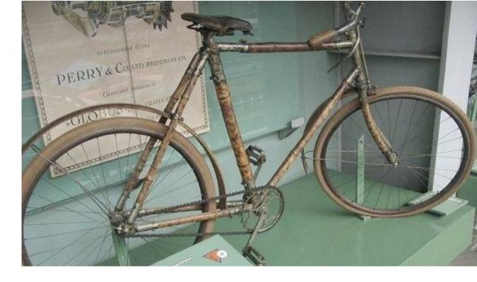
As this bamboo bike from 1896 (in Prague's Technical Museum) shows, bamboo has been used for bike building nearly as long as bikes have been in the mainstream. That's not surprising -- bamboo's lightweight, hollow structure and strength lend itself well to the bike.
